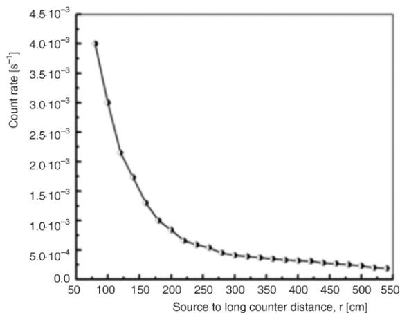
Figure 5. Count rate  $N(r_0)$  vs. distance  $r$  from neutron point source to the long counter front face, for neutron energy at 14 MeV
