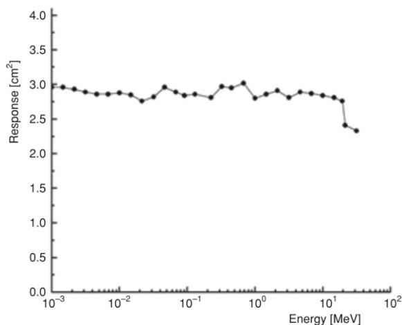
Figure 3. The response function of the designed long counter, calculated from SuperMC code
