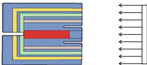
Figure 2. Simulated parallel neutron beam striking the front face of reduced size neutron long counter
