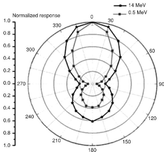
Figure 4. Normalized angular response functions of the reduced size long counter, at 0.5 MeV and 14 MeV neutron energies
