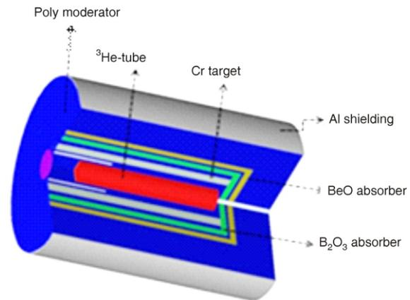
**Figure 1. SuperMC model of the reduced size long counter**
